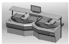
The operators will stand in front of the screen, with retrieved stock delivered on one conveyor. The operator will consolidate the orders and place them on the other conveyor, to be passed on to the packing team before they are dispatched.
